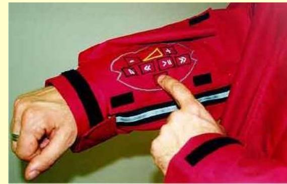
**Quantum Tunnelling Composites (QTC) –** A polymer containing small particles of metal. This material is normally an insulator, but when compressed it becomes a conductor of electricity.
