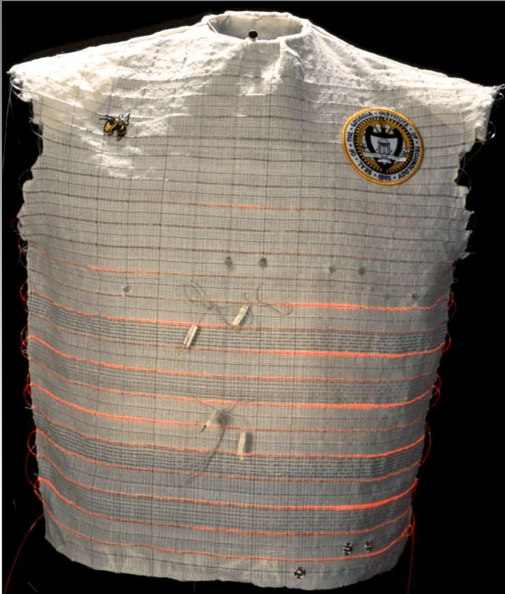
Made of soft, washable fabric, woven with optical and electrical fibres into it, the 'Smart shirt' monitors the wearer's heart rate, body temperature, respiration and a host of other vital functions. The information can be relayed wirelessly to doctors or personal trainers. Future applications include shirts for parental use to monitor babies and for military use to provide a trapped soldier's exact location and give support units exact information about wounds.
