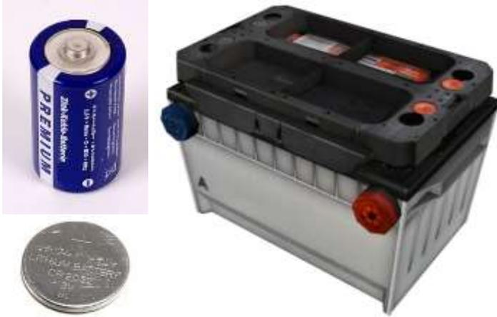
Batteries, like the ones used in torches, watches, calculators and cars, all produce **direct current** (DC). We say it is direct current because it flows in one direction only. When you connect to the red and black terminals on a laboratory power supply, you are using direct current.
