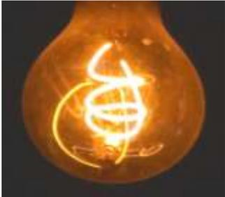
A **filament bulb** is very inefficient. A typical filament bulb has an efficiency of about 20%. That means out of every 100 joules of energy input to it, only 20 joules are transferred as light, which is the useful energy. The other 80 joules are transferred as heat, which is wasted. Filament bulbs don't last very long but they are inexpensive, although it may cost more to replace a filament bulb several times than to buy one of the alternatives that last longer.
