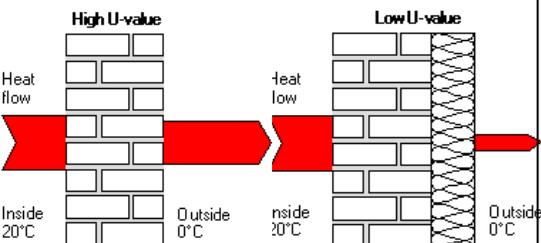
The lower the U-value, the better the material is as an insulator
